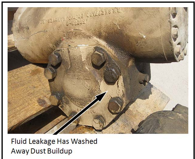
Figure 20: Vehicle Steering Gear Leakage Example
